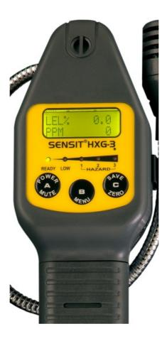
**HINT:** As you approach the source of the leak, keep dialing down the rate of the audible "tick" by dialing down the thumb wheel which is located on the right side of the instrument.
