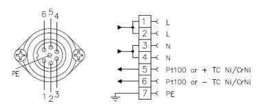
Connector X3 7pole female Heated Sample line (Option)
