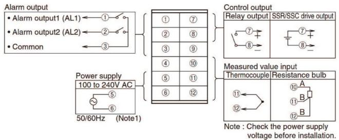
For Pt100 connection shorten pins 11 and 12 and connect sensor between 10 and 11.
