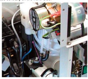
Open nut and remove the sensor downwards. clean and dry the sensor. Dry also the gas path downstream the heat exchanger. check the unti for leaks before starting the operation.
