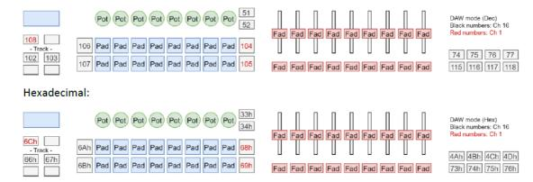
Note that to provide some degree of script compatibility with the Launchkey Mini MK3, the Scene Up and Scene Down buttons also report back CC 68h (104) and 69h (105) respectively on Channel 16.
