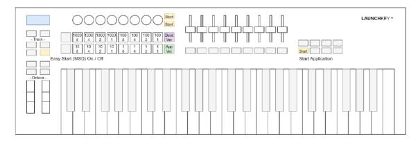
The Launchkey MK3 has a bootloader mode that allows the user to configure and save certain settings. The bootloader is accessed by holding the Octave Up and Octave Down buttons together whilst plugging the device in.
