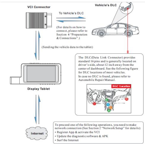
The DLC(Data Link Connector) provides standard 16 pins and is generally located on driver's side, about 12 inch
