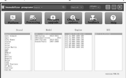
You can also enter relevant information (Brand, Bosch ID or ECU) in the search box to inquire. For example, search for MED17.1 engine through ECU as shown in the figure below.
