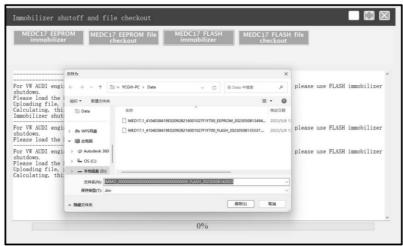
5.1.5 Click EEPROM checkout/FLASH checkout, load the corresponding EEPROM/FLASH backup file as software prompts.
