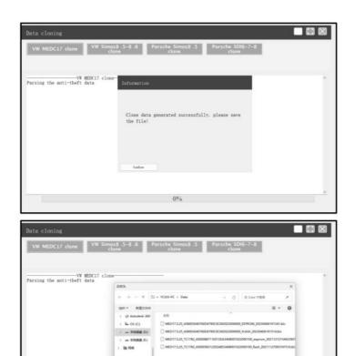
5.2.6 Connect external ECU and ECU&TCU Programmer, write FLASH data of original ECU and saved EEPROM clone data into external ECU.
