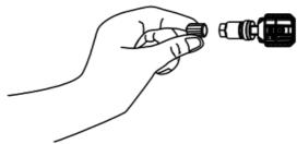
Step 2. Place the valve stem through the valve hole of the rim, ensuring the sensor body located on the inside of the rim. Assemble the nut back on the valve stem with a torque of 4N·m, then tighten the cap.
