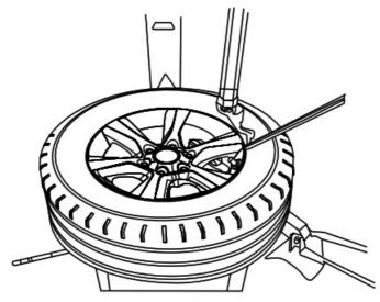
3. Dismounting the sensor Remove the cap and nut from the valve stem, and then remove the sensor assembly from the wheel rim.
