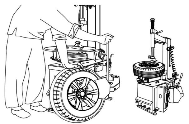
2. Dismounting the tire Clamp the tire on the tire changer, and adjust the valve at 1 o'clock to the tire fitting head. Use the tire tool to dismount the tire bead.
