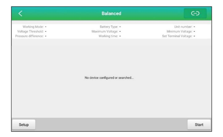
Click "button in the upper right corner of balanced interface to enter the device pairing interface, which can connect with optional devices. "button in the upper right corner of device pairing interface is the clear device pairing button, which deletes all current devices when clicked. If you need to delete a single paired device, long
