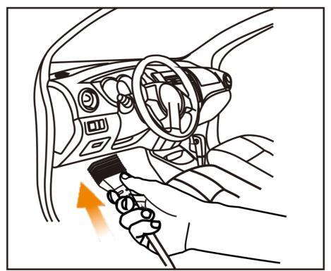
4. Turn on the ignition. Engine can be off or running. Now it is ready for diagnostics.
