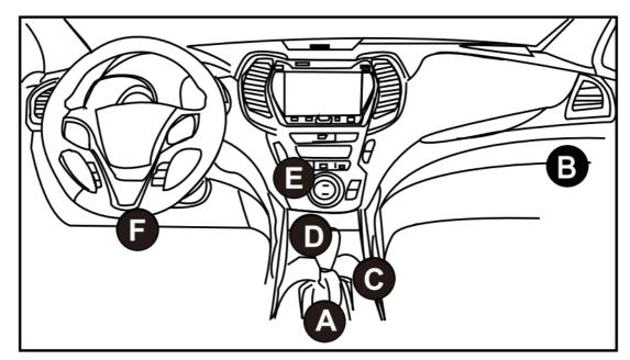
3. Plug the diagnostic cable into vehicle's DLC port.
