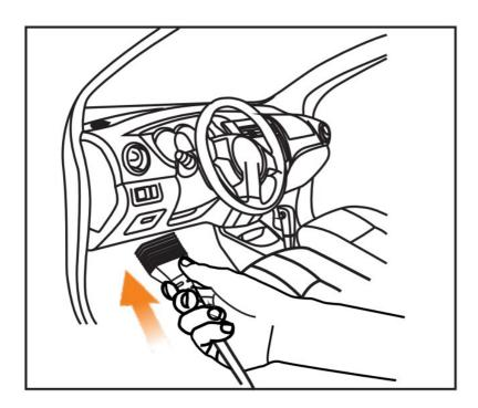
**Note:** For non-OBD II vehicles, a non-16pin connector(adapter cable) is required. Refer to the User Manual for more detailed connection method.
