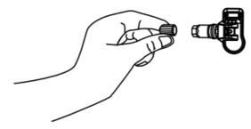
Step 2. Place the valve stem through the valve hole of the rim, ensuring the sensor body is located on the inside of the rim. Assemble the nut back on the valve stem with a torque of 4N·m, then tighten the cap.
