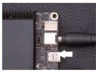
**Step 4:** Connect your keyboard and mouse to the LattePanda Sigma through any of the USB connectors, and connect the power adapter (provided) to the LattePanda Sigma.
