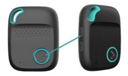
There is no need to turn off the device off unless you will not be using it for a prolonged period of weeks or months. To turn it off, hold down the SOS button and the upper 'Side talk button' together till the device vibrates. Do this twice. The lights will turn off shortly after you feel the vibration. Hold down both buttons together for 2 seconds till the device vibrates and turns off. The LEDS will go out.
