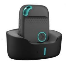
Placing the device in the charging station Please make sure you place the device in the correct position. It is in the correct position when the base light glows. The device is charged when the light turns solid. If the device is off it will turn on when you place it in the charger. Dry device completely before each charge. Wipe all water, sweat, perfumes, and fragrant oils from device before placing in the charging station.
