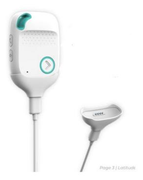
You can charge the device by attaching the magnetic USB-C cable plug to the four charging contacts on the rear of the pendant and the other end into the adapter. Use this charging method when away from home.
