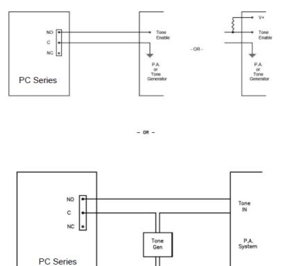
**Important!** Connecting a PC Series clock to a public address (PA) system requires the use of an external Tone Generator. Contact your PA supplier to acquire an appropriate Tone Generator for your system.
