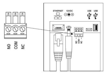
• Connect the wires from the signaling device to the screw terminals. Plug the terminal connector into the socket on the clock. Only one (1) wire should be inserted into the terminal block positions NO and COM, all wire splices should be done externally. See the following diagrams for details.
