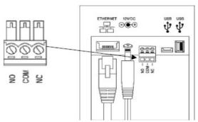
• Connect the wires from the door access device to the screw terminals. Plug the terminal connector into the socket on the PC Series clock. Only one (1) wire should be inserted into the terminal block positions NO and COM, all wire splices should be done externally. See the following diagrams for details.
