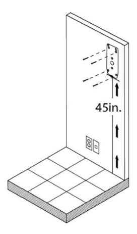
**Note:** The bottom of the clock should be about 45 inches from the floor.
