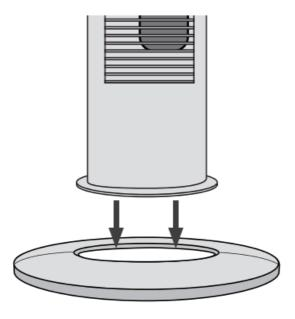
3. Hold the **Body** in place while turning the **Support Base Assembly** clockwise until it no longer turns and locks in place.
