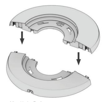
2. Align the Support Base Assembly with the Body.
