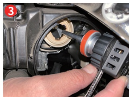
Put the LED into the housing
