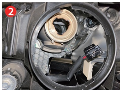
Twist out the halogen bulb
