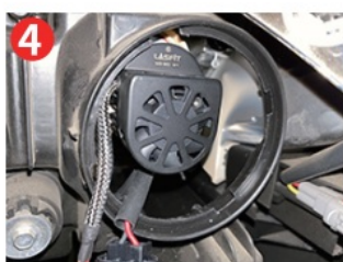
Lock the LED bulb on headlight housing
