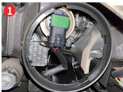
Remove the OEM dust cover
