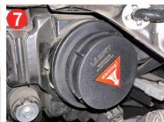
Lock the dust cover with cooling system
