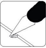
• Use an exact knife to cut the bits connecting the parts to the frame.
