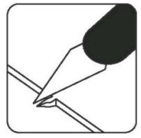
Use an exacto knife to cut the bits connecting the parts to the frame.
