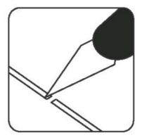
Most joints are press-fit, but some joints might require a drop of glue to ensure a strong bond.
