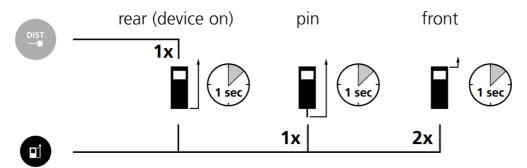
To ensure correct measurements plug-in pin so that it clicks into position!
