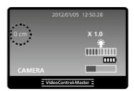
The PipeControl-LevelFlex-Camera features an integrated metre counter. The reeled off number of metres appears on the display of the VideoControl-Master (see image). Settings can be changed by means of the base unit. For more information, see: VideoControl-Master, Section 8.6 Length measure.
