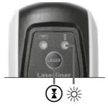
Use an GRX laser receiver (optional) to carry out levelling at great distances or when the laser lines are no longer visible. To work with a laser receiver, switch the line laser to hand-held receiver mode by keeping button 1 (handheld receiver mode on / off) pressed. The laser lines will now pulsate with high frequency, making the laser lines darker. The laser receiver can detect these pulsating laser lines. Observe the laser receiver's operating instructions for line lasers.
