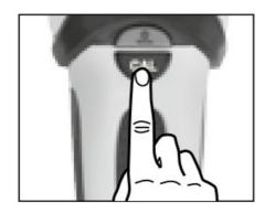
The device and the wall must maintain contact during calibration in STUD-SCAN mode and throughout the entire measurement process. A hand should remain at the device the entire time as well.
