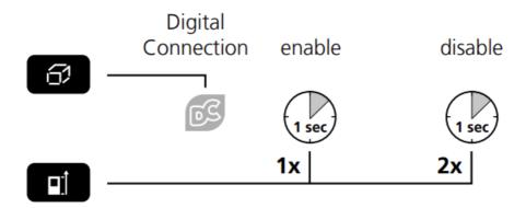
The digital connection is activated as soon as the device is switched on as the wireless system is designed to use very little electricity.
