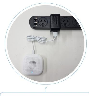
Connect the Gateway to a USB Power Adapter using a Micro USB Cable.
