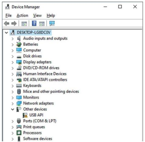
If you expand "Universal Serial Bus Controllers' by clicking the arrow to the left of the text; this is normally where you'd see the logger as "EasyLog USB Device": If your logger is plugged in, but doesn't appear in this list, it is likely under another heading such as other devices. In the example above this shows as "USB API" which indicates the driver has not been installed correctly. This would not be seen by the EL-WIN-USB software because it's an unknown device at this point.
