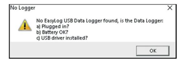
If the logger has not been used for a period of time, a power cycle may be useful, this can be done by removing the battery and re-inserting it after a few seconds. When the battery is inserted, you should get an LED (lamp) flashing sequence for a few seconds followed by no LED's. (Some models may not have visible LED's)
