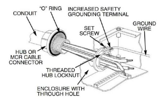
These locknuts must be bonded between each other and to the grounding system using jumper wires. After the entry hardware is installed, connect the appropriate conduit or cable.
