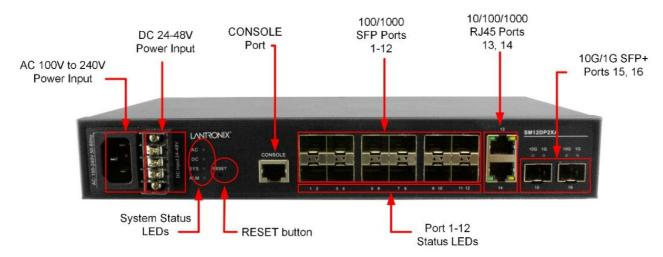
1000BASE-T Ports: The switch contains 10/100/1000BASE-T RJ-45 ports. All RJ-45 ports support automatic MDI/MDI-X operation, auto-negotiation and IEEE 802.3x auto-negotiation of flow control, so the optimum data rate and transmission can be selected automatically.
