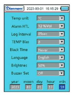
**Notes**: TEMP Bias (Temperature Numerical Compensation Settings) is used to compensate for errors in the measurement process.
