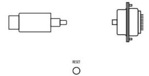
2. Reset button Pressed up to 5 seconds: device restart
