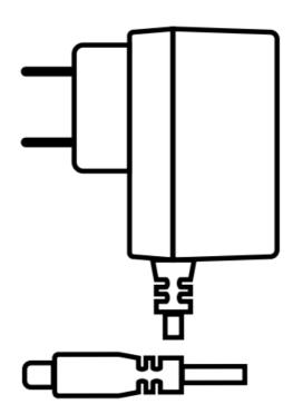
After connecting the cable to the device, turn the connector 90° clockwise to prevent it from accidental un plugging. Use only the supplied power adapter.
