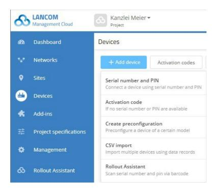
In the next window, enter the serial number and Cloud PIN of the device. Then confirm with the button Add new device.
