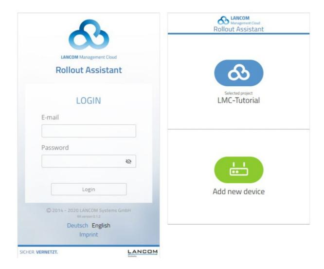
You select the desired language and log in to the LMC using your credentials. On the next page, you select the project that new devices are added to. Do this by tapping the green button and scanning the serial number. The Rollout Assistant may request access to the camera on the device to do this. You scan the serial number either on the underside of the device or alternatively from the barcode on the packaging box. Otherwise, you can enter the serial number manually.
