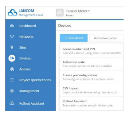
Create an activation code by following the instructions in the dialog. This activation code allows you to integrate the LANCOM device into this project at a later time. The activation code button displays all of the activation codes for this project in the Devices view.
