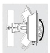
The main beam direction of the integrated antenna can be adjusted by tilting the access point up or down by rotating the connection flange about the mounting arm. Installing access points and/or external antennas without adequate lightning protection can lead to serious damage to the devices and/or to the related network infrastructure
