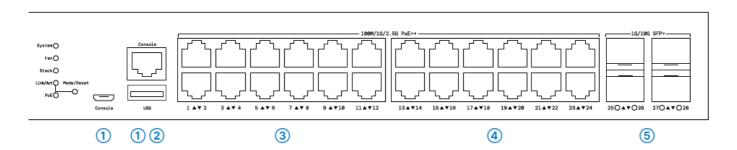
Configuration interfaces RJ-45 & micro USB (Console) Connect the configuration interface via the included micro USB cable to the USB interface of the device you want to use for configuring / monitoring the switch.
