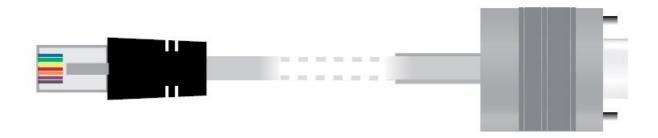
• Connect the configuration interface via the included serial configuration cable to the serial interface of the device you want to use for configuring / monitoring the switch.
