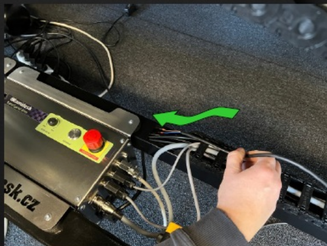
push wiring through tube
