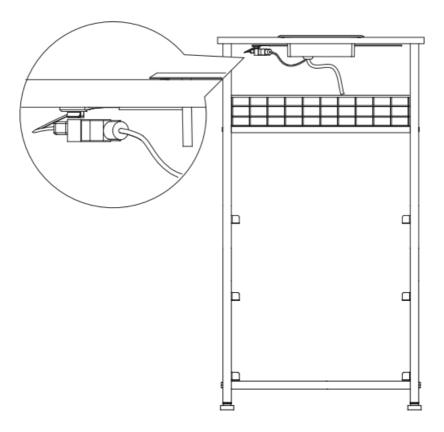
Conect the USB of the LED strip and the USB socket of the outlet  $\,$
