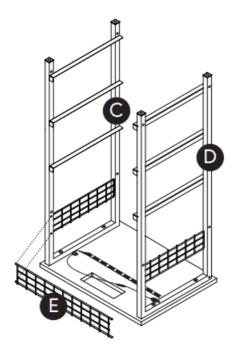
▲ Insert E into the holes in C and D
