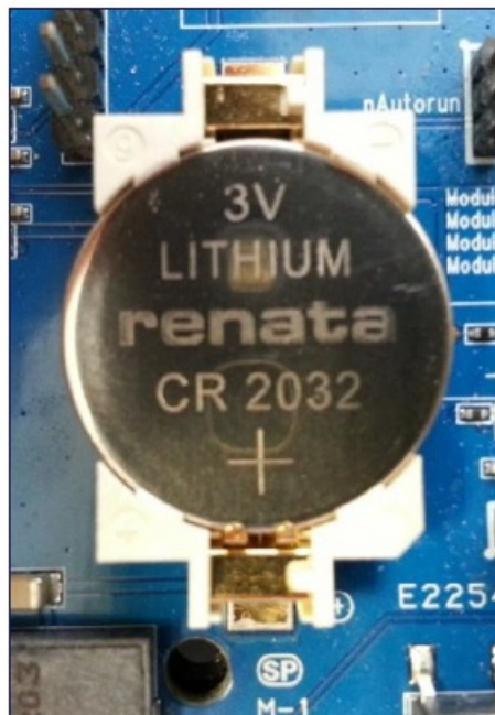
Figure 22: Inserting the coin cell (step 2)
