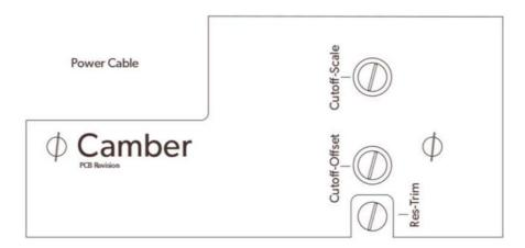
Camber is not calibrated for a voltage per octave response during manufacturing, instead it is adjusted to give the
