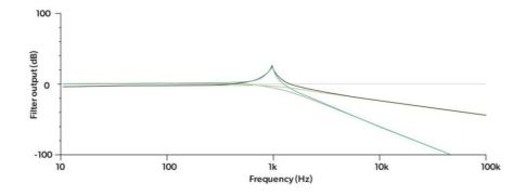
High pass at 1kHz, Brown=One Pole(6dB) Green=Three Pole (18dB)
