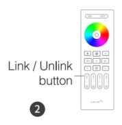
Short press "I" button 5 times within 3 seconds when light on.
