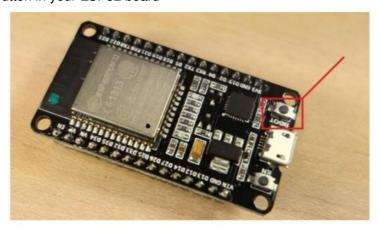
• Press the "Upload" button in the Arduino IDE to upload your sketch:
