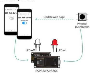
The ESP32 or ESP8266 hosts a web server that allows you to control the state of an output;
