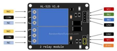
On the left side, there are two sets of three sockets to connect high voltages, and the pins on the right side (low-voltage) connect to the ESP32 GPIOs.
