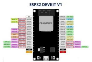
These analog input pins have 12-bit resolution. This means that when you read an analog input, its range may
