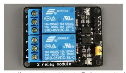
The low-voltage side has a set of four pins and a set of three pins. The first set consists of VCC and GND to power up the module, and input 1 (IN1) and input 2 (IN2) to control the bottom and top relays, respectively. If your relay module only has one channel, you'll have just one IN pin. If you have four channels, you'll have four IN
