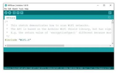
5. Press the Upload button in the Arduino IDE. Wait a few seconds while the code compiles and uploads to your board.
