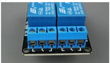
The relay module shown in the previous photo has two connectors, each with three sockets: common (COM), Normally Closed (NC), and Normally Open (NO).
