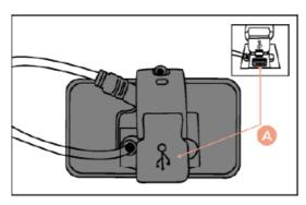
**USB-port** Below the display is a USB port (A) where you can charge, for example, your smartphone or navigation device while cycling. Charging only works when the display is on.
