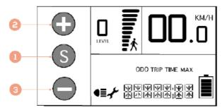
**Thumb lever** By pushing the lever (A) forward when stationary, the walk assist will be activated (which give support up to 6 km/h). Walk assist will be activated when the (-) button is pressed for a few **seconds. Attention:** Walk assist does not work when support mode is set to '0'. Using the lever while pedalling, the support will go to its maximum speed of 25 km/h.
