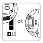
FastPette<sup>™</sup> Pro: Press the SPEED button until the display shows the correct speed – HIGH or LOW. FastPette V2: Change the position of the SPEED switches.
