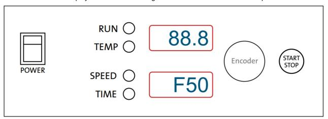
• Press and hold encoder knob for more than 2 seconds. Temperature signal light blinks. With rotating encoder clockwise (+) or counter-clockwise (-), set temperature to desired value: 37.5 = 37.5°C
