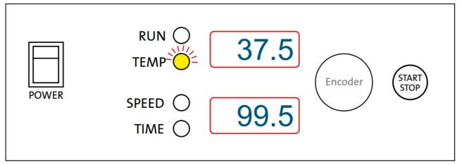
• If you want to use the shaking incubator without temperature regulation set OFF on display. You get OFF function on display, when you rotate encoder under 0.0°C or above 70.0°C.
