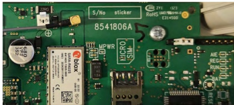
Picture 6 The antenna is connected to the MMCX connector above the radio module
