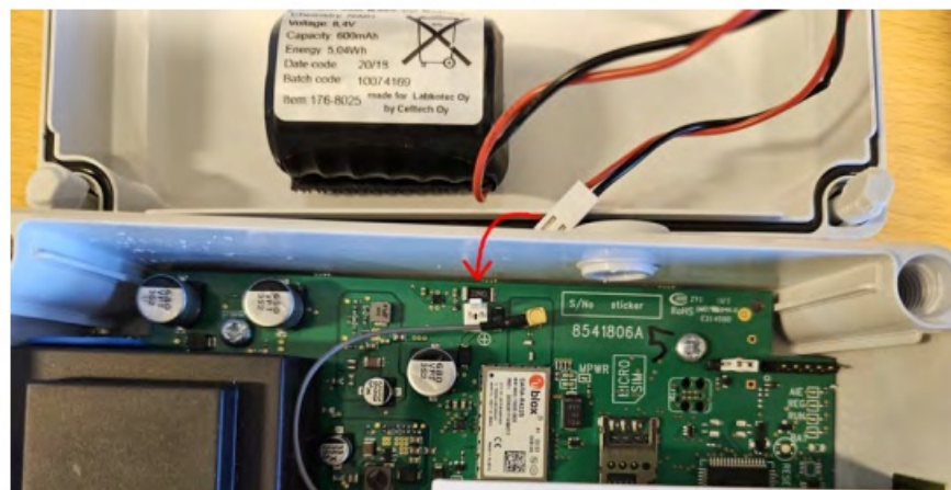
Figure 4: Connecting the battery backup to Labcom 442.
