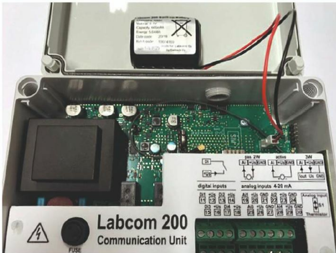
Figure 21 . Connecting the Labcom 200 battery backup.
