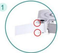
Tum the green gear in the direction of arrow on the tape until tight to tighten the carbon ribbon.
