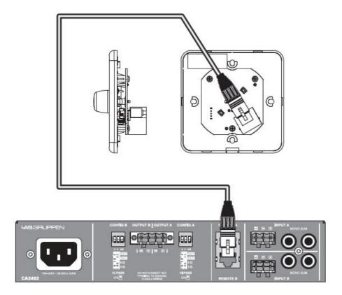
Wire the CRC-VEU to any Remote port on a CA, CM, CMA and CPA product to control the volume of the channel associated with the Remote port. With custom cabling, a single remote can also be paralleled to the other channels' remote port on a two-channel device.
