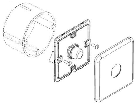
The CRC-VEU fastens into the installation enclosure with two screws beneath the front plate. Remove the front panel, and fasten the main unit into the enclosure with the mounting screws from the enclosure. When the unit is securely fastened, replace the front panel.
