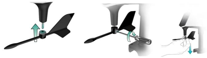
2. Carefully tighten the screw on the side of the vane using a mini screwdriver. The screw should tighten into the flat edge of the post. When the screw is tight, gently pull on the vane to ensure it is secure.
