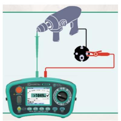
PAT test (PAT = Portable Appliance Tester) It is possible to check the insulation resistance and earth bond continuity of portable appliances for class I and II.
