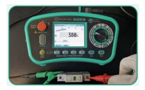
SPD (Surge Protection Device) which contains varistor can be tested measuring the tripping voltage without damage it.
