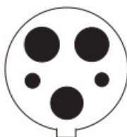
KEW 8601 EVSE ADAPTER TYPE1 plug
